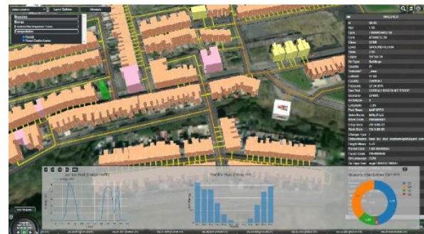
Figure A4: User interface – typical daily household heat energy profile, monthly and quarterly heat energy requirements
