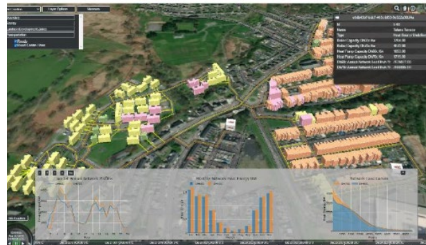
Figure A2: User interface – energy centre network profiles, monthly heat energy supply and load curves
