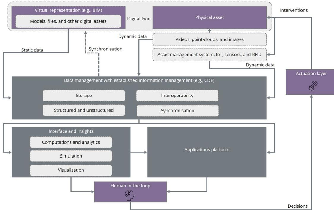
Figure 4: Components of a digital twin
