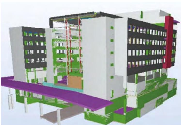
Image: EQUA Sensus system applied to Fennia Office Building, Helsinki renovation. Ceiling heating/cooling panels, integrated to Sensus-system, were carefully dimensioned and positioned, resulting in improved comfort and 25-35% energy savings compared to the tradition system.
